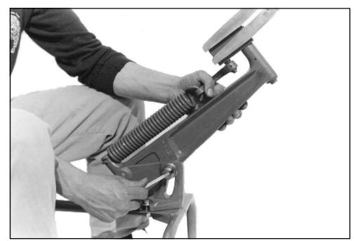
The photographs to the right show a Super Trap 3 being adjusted for elevation. The procedure is identical on the Super Trap 2000.
